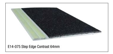
The E14-075 Step Edge Contrast is designed to ensure visibility of steps in escape routes to meet NZBC Clause F6 "Visibility in Escape Routes". The Step Edge contrast will be effective in all light conditions including during failure of the main lighting.
